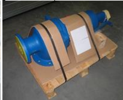
Figure 6.2.13-2: Tied-down on a pallet
