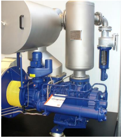
Figure 6.2.5.3-1: LESER Safety Valves in the non-upright position
