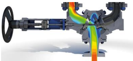
Figure 6.6.2.2-1: Enhanced flow path
