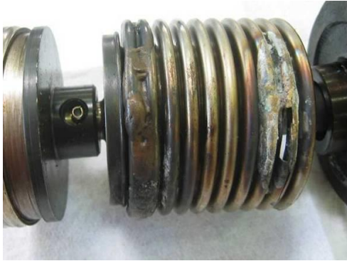
Figure 17.3.5-1: Symptom 16 - Corroded stainless steel bellows
